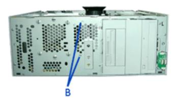
Figure 4 - 20 : HDD Bracket Screws
